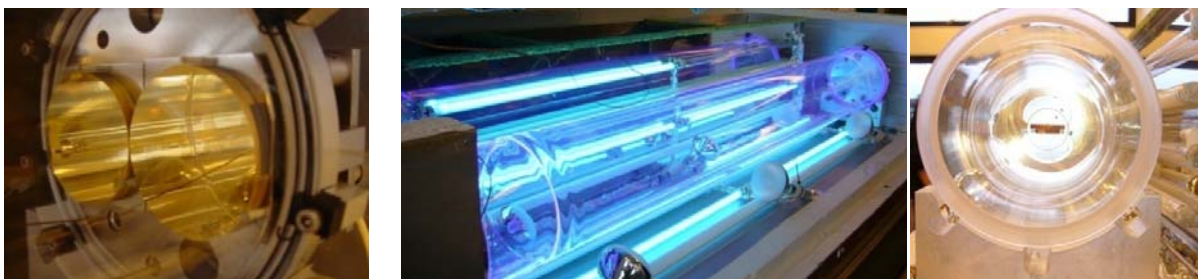
Figure 3. The photochemical reactor. System components pictured include custom gold-coated multipass optics, solid quartz reaction cylinder, double O-ring sealing of end flanges, lamp systems and temperature control housing.
